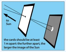
A simple yet safe way to view the solar eclipse is by making a pinhole viewer.
