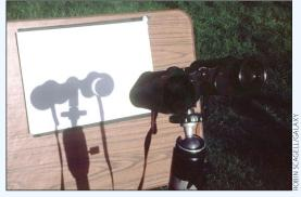
Sun drifts out of the field of view, it might melt the inside of the eyepiece! So take great care, or use an old eyepiece (many older eyepieces used metal rather than plastic).
